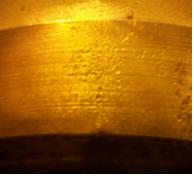
On the left was a 27" flange face. This face had many imperfections, some of which was damage. Metal Surgery Milwaukee LTD. made a clean up cut, then the phonographic finish cut. These repairs were made in minimal time allowing the customer to keep his shipping deadline.
