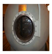
Flange facing may be needed in a numerous number of parts such as these boiler tanks. Metal Surgery Milwaukee LTD. has capabilities of flange facing up to 120". Below are two different boiler tanks which needed flange facing due to imperfections and slight damage to the finish. These parts required a phonographic finish.
